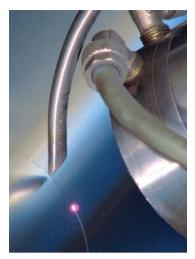
Our patented, overlap-free laser welding process allows sheets of up to 1500 mm without leakage channels.
