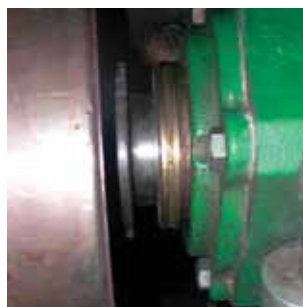
LabTecta-AX™ installed on a paper machine roll (Case Ref: 3482)
