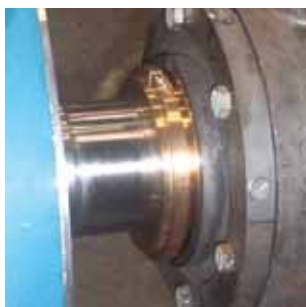
LabTecta-AX™ installed on a breast roll (Case Ref: 3326)
