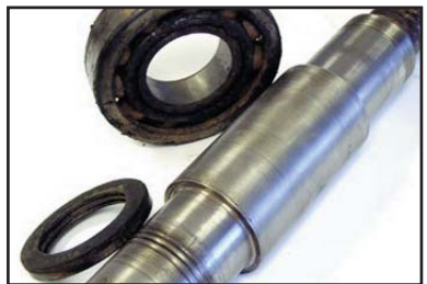
Shaft damage from a Labyrinth Seal.
