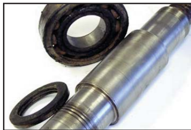
Shaft damage from a Labyrinth Seal.
