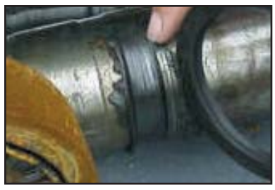
Shaft damage from Lip Seals.
