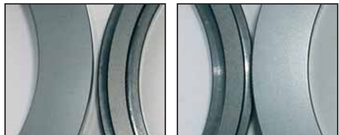
100mm (4.000") EASASEAL™ faces after 500 hours testing at 100 bar (1500 psi).
